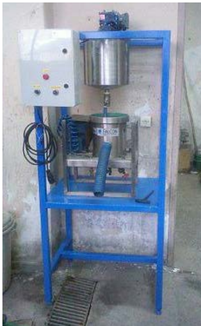
Fig. 2. The L-40 Laboratory Scale Falcon Concentrator
