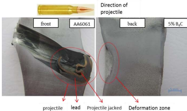
Figure 6. Sample with 7.62 × 51 mm bullet shot with G3 rifle placed side by side after extrusion
